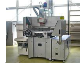
Manufacturer: Kuroda Precision Industries Ltd Model: Forming Surface Grinding Machine Model Number: GS-45 Donor: Kuroda Precision Industries Ltd.
