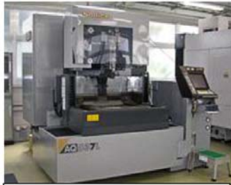
Manufacturer: Sodick Co., Ltd. Model: Linear Motor Drive Wire-Cut EDM Model Number: AQ537L Donor: Sodick Co., Ltd.
