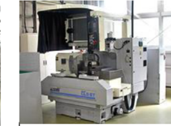
Manufacturer: Techno Washino Model: Optical Precision Profile Grinder Model Number: GLS-5T Donor: Techno Washino
