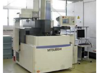
Manufacturer: Mitsubishi Electric Corporation Model: Die-Sinking EDM Model Number: EA12/E Donor: Mitsubishi Electric Corporation
