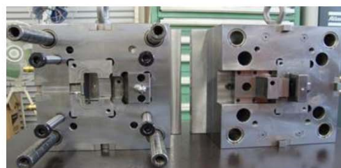
Left: Completed product (tea bag rest) Center: Injection molding Right: Mold dies
